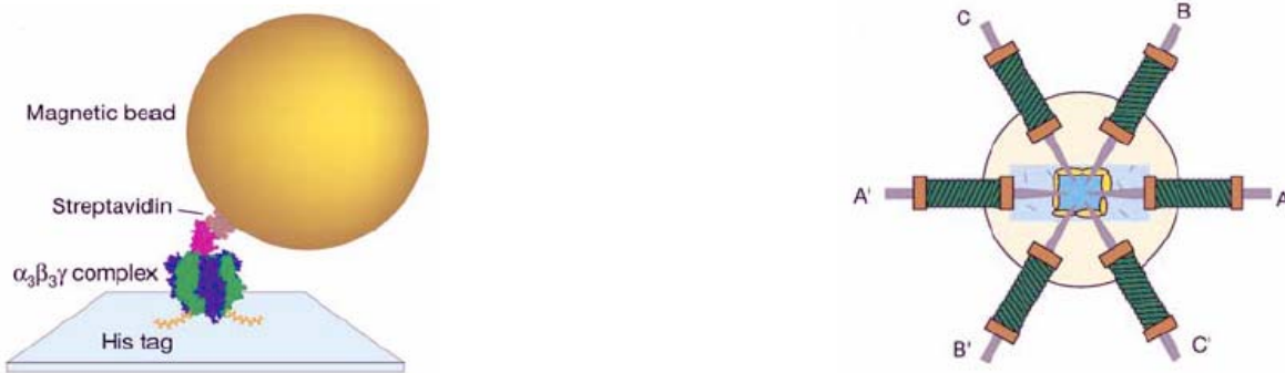
Figure 7: Magnetic bead is attached to the \gamma subunit here (left figure) and the arrangement of the magnets (right figure) [Ref: 76]
